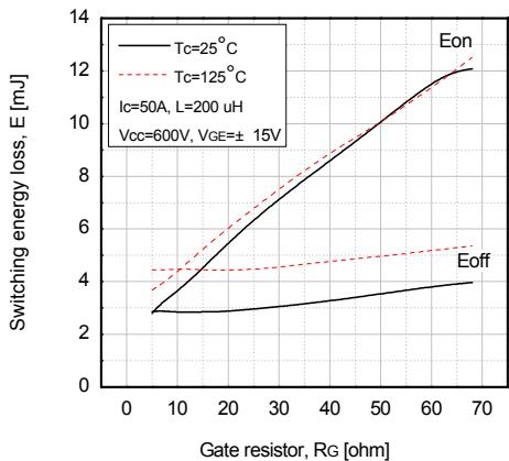
**Fig 8. Typical switching loss vs gate resistor**
