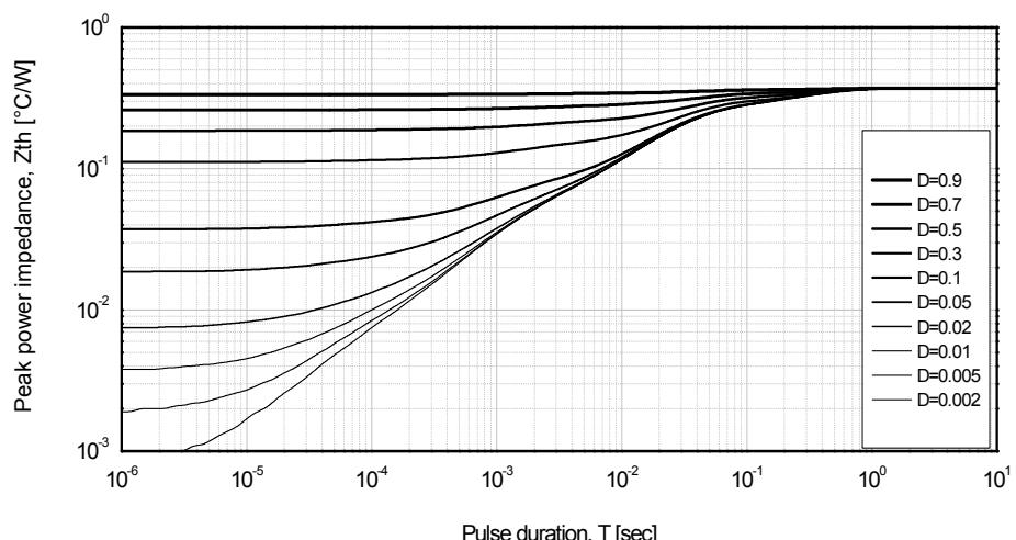
**Fig 13. IGBT transient thermal impedance**
