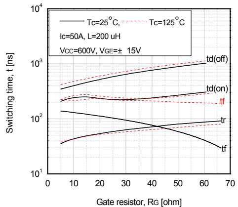
**Fig 7. Typical switching time vs gate resistor**
