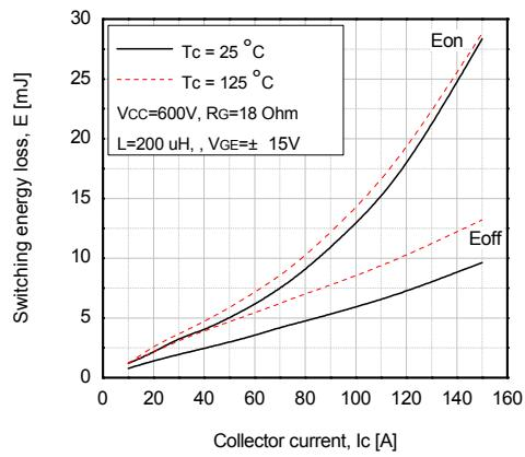
**Fig 6. Typical switching loss vs collector current**
