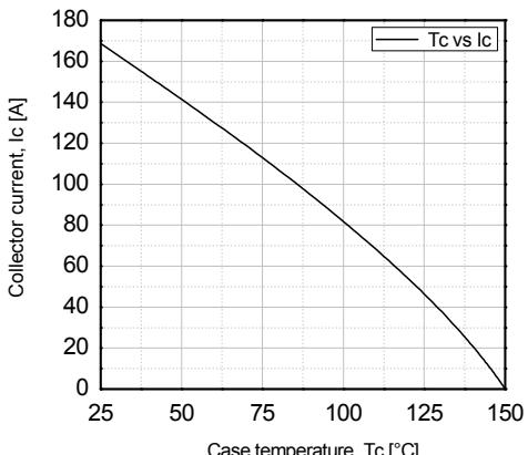
**Fig 11. Case temperature vs collector current**
