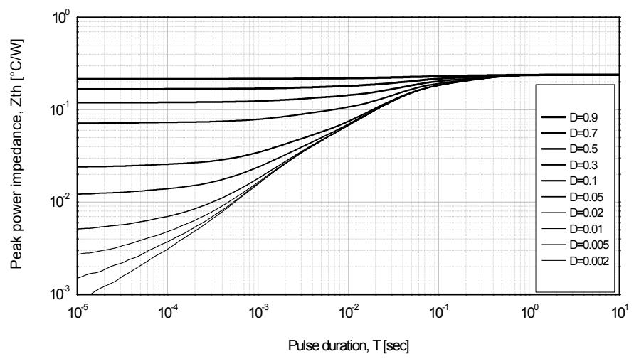
**Fig 13. IGBT transient thermal impedance**
