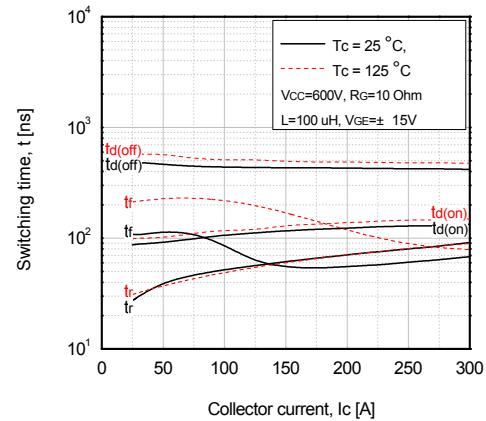
**Fig 5. Typical switching time vs collector current**
