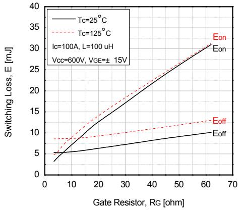
**Fig 8. Typical switching loss vs gate resistor**
