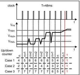
Figure 5 Up/down counter operation
