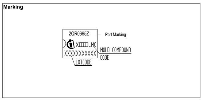
Figure 15 Marking for ICE2QR0665Z
