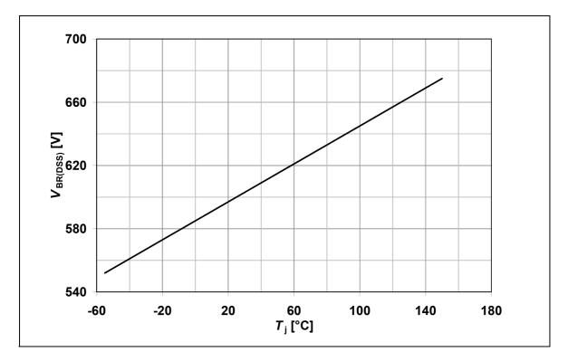
Figure 11 Drain-source breakdown voltage;  $V_{BR(DSS)}=f(T_j)$
