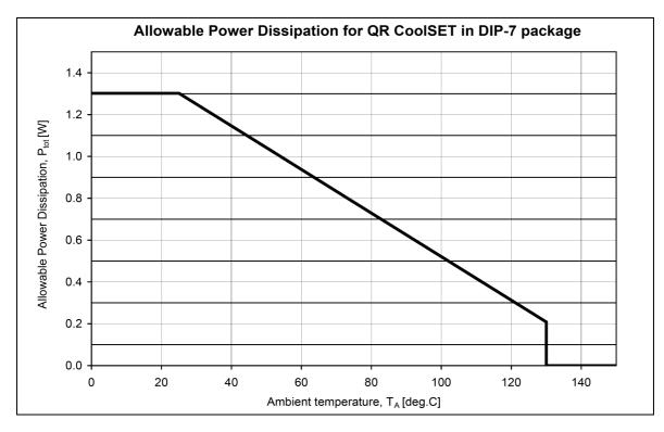
Figure 10 Power dissipation;  $P_{tot}=f(T_a)$
