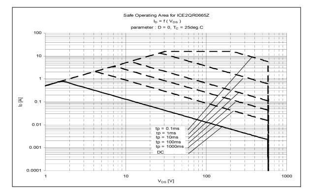
Figure 9 Safe Operating Area(SOA) curve for ICE2QR0665Z
