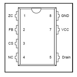
Figure 1 Pin Configuration PG-DIP-7 (top view)
