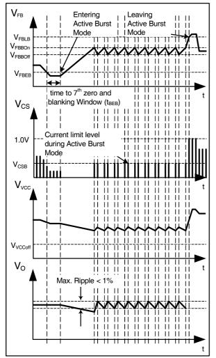
Figure 8 Signals in Active Burst Mode
