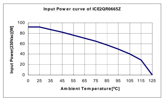
Figure 13 Input Power curve  $Vin=230Vac;Pin=f(T_a)$
