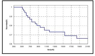
Figure 7  $V_{CS-max}$  versus  $I_{ZC}$
