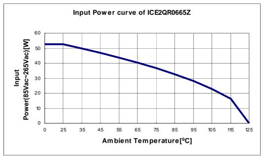
Figure 12 Input Power curve Vin= $85 \sim 265$ Vac;Pin= $f(T_a)$
