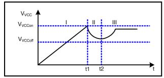
Figure 3 VCC voltage at start up
